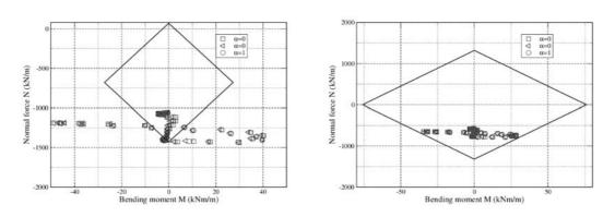
Fig. 10. Bending moment vs. normal force for shotcrete (left) and steel ribs (right) (case 2)
