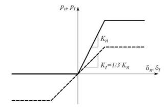
Fig. 2. Constitutive relationship of the springs representing the ground reaction in the bedded-spring model  $p_n$  and  $p_t$  represent the normal and tangential load,  $\delta_n$  and  $\delta_n$  the normal and tangential displacement and  $K_n$  and  $K_t$  the normal and tangential stiffness
