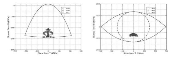
Fig. 11. Shear force vs. normal force for shotcrete (left) and steel ribs (right) (case 2). In the right figure the dotted ellipse represent the Tresca criterion while the solid curve represent the maximum strength criterion
