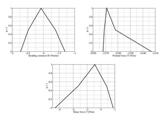
Fig. 6. Membership functions for bending moment, normal force and shear force (element 48) for case 1
