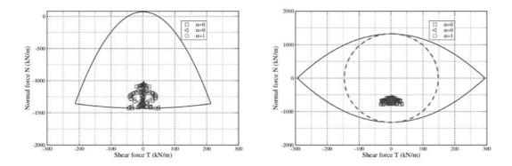
Fig. 9. Shear force vs. normal force for shotcrete (left) and steel ribs (right) (case 1). In the right figure the dotted ellipse represent the Tresca criterion while the solid curve represent the maximum strength criterion
